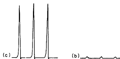
Fig. 5. Analysis of gingival crevice fluid using FIA. Pre-injection phase, No. 1 in Table I; post-injection phase, PC-B (pH 10); excitation wavelength, 392 nm, emission wavelength, 616 nm. (a) Subject given tetracycline orally; (b) subject not given tetracycline. Sensitivity in (b) 10\times greater than in (a).
